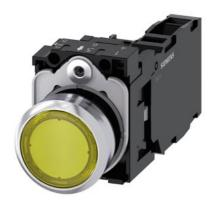
Illuminated pushbutton, 22 mm, round, metal, shiny, yellow, pushbutton, flat, momentary contact type, with holder, 1 NO+1 NC, LED module with integrated LED 24 V AC/DC, screw terminal
