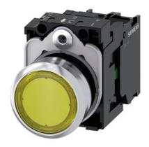
Illuminated pushbutton, 22 mm, round, metal, shiny, yellow, pushbutton, flat, momentary contact type, with holder, 1 NO, LED module with integrated LED 24 V AC/DC. screw terminal
