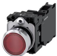
Illuminated pushbutton, 22 mm, round, metal, shiny, red, pushbutton, flat, momentary contact type, with holder, 1 NO+1 NC, LED module with integrated LED 24 V AC/DC, Spring-type terminal
