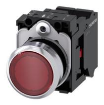
Illuminated pushbutton, 22 mm, round, metal, shiny, red, pushbutton, flat, momentary contact type, with holder, 1 NC, LED module with integrated LED 24 V AC/DC, Spring-type terminal
