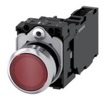
Illuminated pushbutton, 22 mm, round, metal, shiny, red, pushbutton, flat, momentary contact type, with holder, 1 NO+1 NC, LED module with integrated LED 24 V AC/DC, screw terminal
