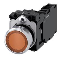
Illuminated pushbutton, 22 mm, round, metal, shiny, amber, pushbutton, flat, momentary contact type, with holder, 1 NO+1 NC, LED module with integrated LED 24 V AC/DC, screw terminal
