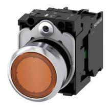
Illuminated pushbutton, 22 mm, round, metal, shiny, amber, pushbutton, flat, momentary contact type, with holder, 1 NO, LED module with integrated LED 24 V AC/DC. screw terminal
