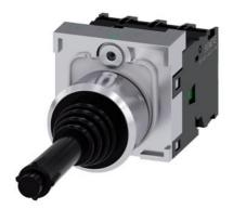
Coordinate switch, 22 mm, round, metal shiny, black, 4 switch positions, latching, with mechanical interlocking, in O position, with holder, 1 NO, 1 NO, 1 NO, 1 NO, screw terminal.
