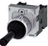
Coordinate switch, 22 mm, round, metal shiny, black, 2 switch positions, horizontal latching, with mechanical interlocking, in O position, with holder, 1 NO, 1 NO, screw terminal,
