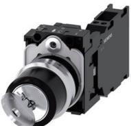
RONIS key-operated switch, 22 mm, round, metal, shiny, lock number SB30, with 2 keys, 2 switch positions O-I, latching, actuating angle 90°, 10:30h/13:30h, key removal O+I, with holder, 1 NO+1 NC, spring-type terminal, possible special locks: SB31, 421, 455
