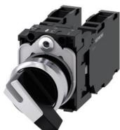
Toggle switch, 22 mm, round, metal, shiny, white, knob, long, 2 switch positions O-I, latching, actuating angle  $90^{\circ}$ , 10:30h/13:30h, with holder, 1 NO, 1 NO, screw terminal
