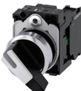
Toggle switch, 22 mm, round, metal, shiny, white, knob, long, 2 switch positions O-I, latching, actuating angle  $90^{\circ}$ , 10:30h/13:30h, with holder, 1 NO, screw terminal
