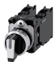
Selector switch, illuminable, 22 mm, round, metal, shiny, white, selector switch, short, 3 switch positions I>O<II, momentary contact type, actuating angle 2x45°, 10:30h/12h/13:30h, with holder, 2x1NO+1NC, Spring-type terminal
