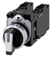
Selector switch, illuminable, 22 mm, round, metal, shiny, white, selector switch, short, 3 switch positions I>O<II, momentary contact type, actuating angle 2x45°, 10:30h/12h/13:30h, with holder, 2x1NO+1NC, screw terminal
