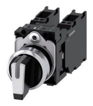
Selector switch, illuminable, 22 mm, round, metal, shiny, white, selector switch, short, 3 switch positions I-O-II, latching, actuating angle 2x45°, 10:30h/12h/13:30h, with holder, 2x1NO+1NC, Spring-type terminal
