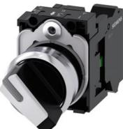
Selector switch, illuminable, 22 mm, round, metal, shiny, white, selector switch, short, 2 switch positions O-I, latching, actuating angle 90°, 10:30h/13:30h, with holder, 1 NO, Spring-type terminal
