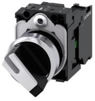
Toggle switch, 22 mm, round, metal, shiny, white, knob, short, 2 switch positions O<I, momentary contact type, actuating angle  $45^\circ$ , 10:30h/12h, with holder, 1 NO, screw terminal
