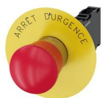
EMERGENCY STOP mushroom pushbutton, 22 mm, round, metal, shiny, red, 40 mm, positive latching, acc. to EN ISO 13850, rotate-to-unlatch, with yellow backing plate, inscription: Arrêt d'urgence, with holder, 1 NO+1 NC, screw terminal
