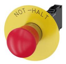
EMERGENCY STOP mushroom-type actuator, 22 mm, round, metal, shiny, red, 40 mm, positive latching, according to EN ISO 13850, rotate-to-unlatch, with yellow backing plate, inscription: NOT-HALT, with holder, 1 NO+1 NC, screw terminal
