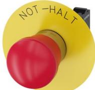
EMERGENCY STOP mushroom-type actuator, 22 mm, round, metal, shiny, red, 40 mm, positive latching, according to EN ISO 13850, pull-to-unlatch mechanism, with yellow backing plate, inscription: NOT-HALT, with holder, 1 NC, 1 NC, spring-type terminal
