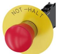
EMERGENCY STOP mushroom-type actuator, 22 mm, round, metal, shiny, red, 40 mm, positive latching, according to EN ISO 13850, pull-to-unlatch mechanism, with yellow backing plate, inscription: NOT-HALT, with holder, 1 NO+1 NC, spring-type terminal
