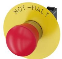
EMERGENCY STOP mushroom-type actuator, 22 mm, round, metal, shiny, red, 40 mm, positive latching, according to EN ISO 13850, pull-to-unlatch mechanism, with yellow backing plate, inscription: NOT-HALT, with holder, 1 NC, spring-type terminal
