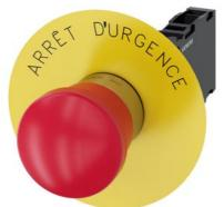
EMERGENCY STOP mushroom pushbutton, 22 mm, round, metal, shiny, red, 40 mm, positive latching, acc. to EN ISO 13850, pull-to-unlatch mechanism, with yellow backing plate, inscription: Arrêt d'urgence, with holder, 1 NO+1 NC, screw terminal
