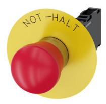
EMERGENCY STOP mushroom-type actuator, 22 mm, round, metal, shiny, red, 40 mm, positive latching, according to EN ISO 13850, pull-to-unlatch mechanism, with yellow backing plate, inscription: NOT-HALT, with holder, 1 NO+1 NC, screw terminal
