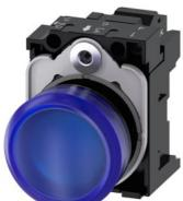
Indicator lights, 22 mm, round, plastic, blue, lens, smooth, with holder, LED module, with integrated LED 230 V AC, Spring-type terminal
