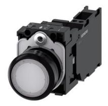
Illuminated pushbutton, 22 mm, round, plastic, white, pushbutton, flat, momentary contact type, with holder, 1 NO+1 NC, LED module with integrated LED 230 V AC, Spring-type terminal
