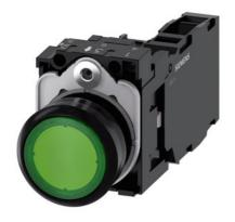
Illuminated pushbutton, 22 mm, round, plastic, green, pushbutton, flat, momentary contact type, with holder, 1 NO+1 NC, LED module with integrated LED 230 V AC, screw terminal
