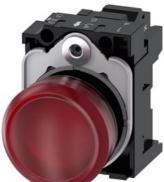
Indicator lights, 22 mm, round, plastic, red, lens, smooth, with holder, LED module with integrated LED 110 V AC, Spring-type terminal
