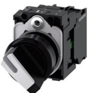
Selector switch, illuminable, 22 mm, round, plastic, white, knob, short, 2 switch positions O-I, latching, 10:30 / 13:30, with holder, with LED module, green, with integrated LED 110 V AC, 1 NO, screw terminal
