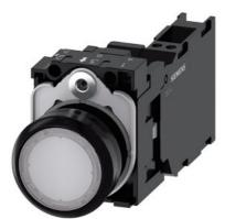
Illuminated pushbutton, 22 mm, round, plastic, white, pushbutton, flat, momentary contact type, with holder, 1 NO+1 NC, LED module with integrated LED 110 V AC, Spring-type terminal
