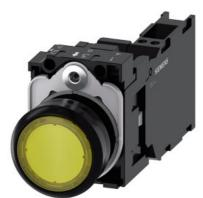
Illuminated pushbutton, 22 mm, round, plastic, yellow, pushbutton, flat, momentary contact type, with holder, 1 NO+1 NC, LED module with integrated LED 110 V AC, Spring-type terminal
