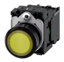
Illuminated pushbutton, 22 mm, round, plastic, yellow, pushbutton, flat, momentary contact type, with holder, 1 NO, LED module with integrated LED 110 V AC, screw terminal
