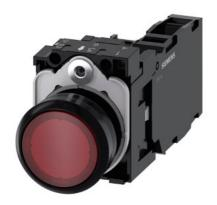
Illuminated pushbutton, 22 mm, round, plastic, red, pushbutton, flat, momentary contact type, with holder, 1 NO+1 NC, LED module with integrated LED 110 V AC, screw terminal
