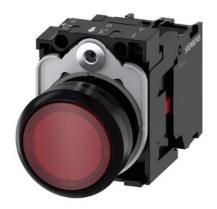
Illuminated pushbutton, 22 mm, round, plastic, red, pushbutton, flat, momentary contact type, with holder, 1 NC, LED module with integrated LED 110 V AC, screw terminal
