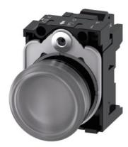
Indicator lights, 22 mm, round, plastic, clear, lens, smooth, with holder, LED module, with integrated LED 24 V AC/DC, Spring-type terminal
