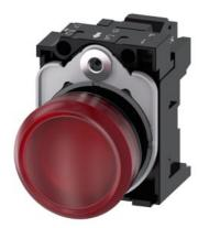
Indicator lights, 22 mm, round, plastic, red, lens, smooth, with holder, LED module, with integrated LED 24 V AC/DC, Spring-type terminal
