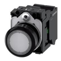
Illuminated pushbutton, 22 mm, round, plastic, clear, pushbutton, flat, momentary contact type, with holder, 1 NO, LED module with integrated LED 24 V AC/DC, Spring-type terminal
