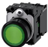
Illuminated pushbutton, 22 mm, round, plastic, green, pushbutton, flat, momentary contact type, with holder, 1 NO, LED module with integrated LED 24 V AC/DC, screw terminal
