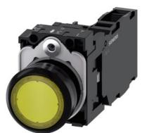
Illuminated pushbutton, 22 mm, round, plastic, yellow, pushbutton, flat, momentary contact type, with holder, 1 NO+1 NC, LED module with integrated LED 24 V AC/DC, screw terminal
