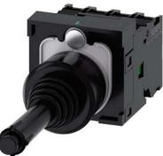
Coordinate switch, 22 mm, round, plastic, black, 4 switch positions, momentary contact type, with mechanical interlocking in O position, with holder, 1 NO, 1 NO, 1 NO, 1 NO, screw terminal
