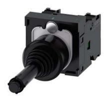
Coordinate switch, 22 mm, round, plastic, black, 2 switch positions, horizontal, momentary contact type, with mechanical interlocking in O position, with holder, 1 NO, 1 NO, screw terminal
