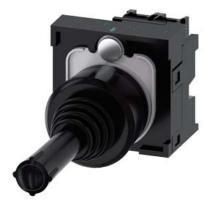
Coordinate switch, 22 mm, round, plastic, black, 2 switch positions, vertical latching, without mechanical interlocking, in O position, with holder, 1 NO, 1 NO, screw terminal
