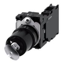
key-operated switch Siemens, 22 mm, round, plastic, lock number SSG10, with 2 keys, 2 switch positions O-I, latching, 10:30h/13:30h, key removal O+I, with holder, 1 NO+1 NC, spring-loaded terminal
