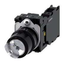
RONIS key-operated switch, 22 mm, round, plastic, lock number SB30, with 2 keys, 2 switch positions O-I, latching, 10:30h/13:30h, with holder, 2 x 1 NC with mounting monitoring, spring-type terminal, possible special locks: SB31, 421, 455
