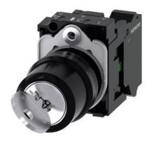
RONIS key-operated switch, 22 mm, round, plastic, lock number SB30, with 2 keys, 2 switch positions O-I, latching, 10:30h/13:30h, key removal O+I, with holder, 1 NO, spring-type terminal, possible special locks: SB31, 421, 455
