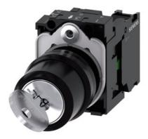
RONIS key-operated switch, 22 mm, round, plastic, lock number SB30, with 2 keys, 2 switch positions O-I, latching, 10:30h/13:30h, key removal O+I, with holder, 1 NO, screw terminal, possible special locks: SB31, 421, 455
