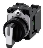
Selector switch, illuminable, 22 mm, round, plastic, white, selector switch, short, 3 switch positions I-O-II, latching, 10:30h/12h/13:30h, with holder, 1 NO, 1 NO, Spring-type terminal
