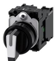
Selector switch, illuminable, 22 mm, round, plastic, white, selector switch, short, 3 switch positions I-O-II, latching, 10:30h/12h/13:30h, with holder, 1 NO, 1 NO, screw terminal
