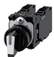
Selector switch, illuminable, 22 mm, round, plastic, white, selector switch, short, 3 switch positions I-O-II, latching, 10:30h/12h/13:30h, with holder, 2x1NO+1NC, screw terminal
