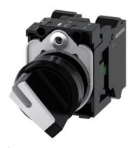
Selector switch, illuminable, 22 mm, round, plastic, white, selector switch, short, 2 switch positions O-I, latching, 10:30h/13:30h, with holder, 1 NO, 1 NC, Spring-type terminal
